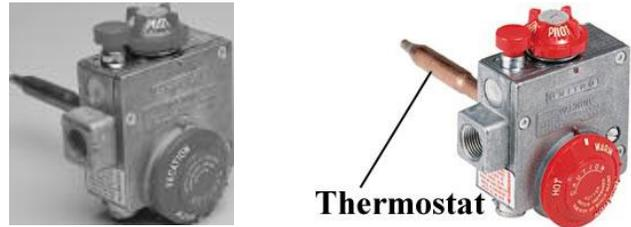
If Gas control valve senses temperatures over 180°F, it will trip **ECO fuse** located inside gas control valve. Many water heaters require replacement of gas valve after thermal event. Other gas water heaters have re-settable thermal switch with wires leading to valve.
