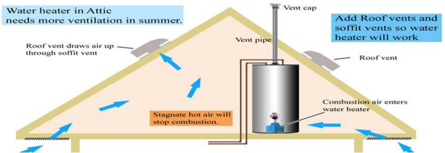
Attics, basements, closets need adequate incoming air supply. Very hot air in attic will cause oxygen molecules to separate and no longer support pilot flame. Open doors and windows, and add vents to get air to water heater. Backdraft and tight house, furnace, fireplace, and other gas appliances that draw air etc, can combine with mechanical vent fans such as range hood, bathroom fans, to create negative pressure inside house that blows out pilot light.
