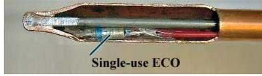
**\*\* ECO: WATER TEMPERATURES IN EXCESS OF 180° F WILL CAUSE HIGH LIMIT CONTROL (ECO) TO OPEN AND SHUT OFF GAS SUPPLY TO UNIT. THE HIGH LIMIT CONTROL IS A SINGLE USE TYPE THAT WILL REQUIRE REPLACEMENT OF THERMOSTAT BEFORE THE BURNER CAN OPERATE.**
